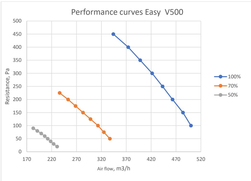
Graph 5 Dependence of ventilation power on the resistance of the installed ventilation system
