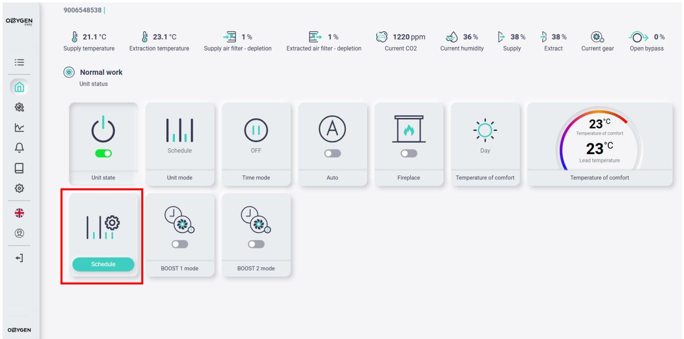
After pressing this button, a window for compiling a weekly program will appear. In it, according to the most suitable need for you, you will be able to arrange a weekly schedule of operation of the device. After the schedule is drawn up for each day, click on the "Accept" button at the bottom of the window.
