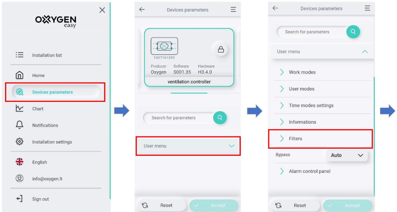
In the tab "Start filter change procedure" we select "Yes". After a few seconds, you will see the "Filter change procedure" section. Expand it and select the filter class that will be use and press "Accept". Then, one by one, we confirm that we have changed the filter. After these steps, "Has filter change was completed" will appear, press and select "Yes". The filter replacement process is complete.
