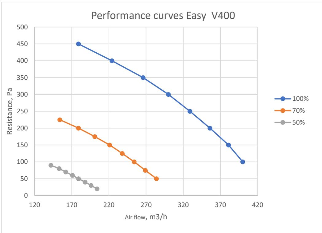
Graph 3 Dependence of ventilation power on the resistance of the installed ventilation system
