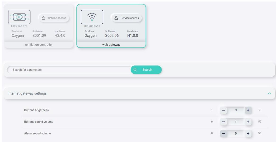
In the **Ventilation controller** window, the **user menu** drop-down list allows you to see details about the device and perform various configuration actions. A detailed description of "User menu" is in Table 6, point 5.4.
