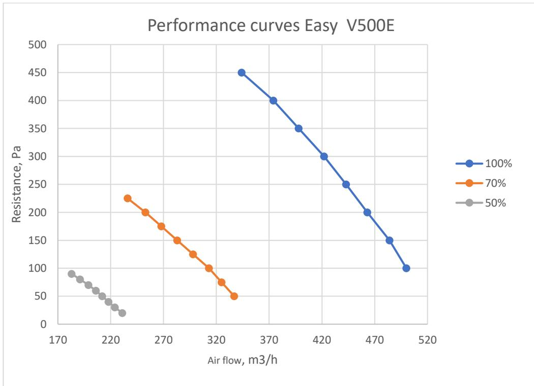
Graph 6 Dependence of ventilation power on the resistance of the installed ventilation system
