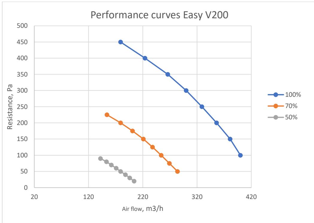
Graph 2 Dependence of ventilation power on the resistance of the installed ventilation system
