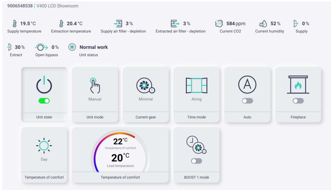
**Auto** – the device will work according to the data received by the humidity and CO2 (if installed) sensor. With an increase in humidity levels or CO2 levels, the unit will easily increase its speed until it reaches the established norms.
