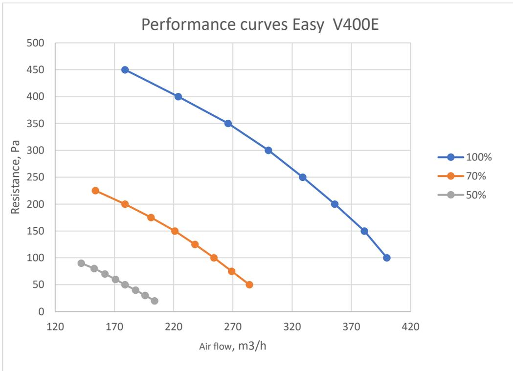
Graph 4 Dependence of ventilation power on the resistance of the installed ventilation system
