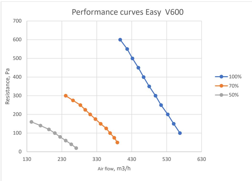
*Graph 7 Dependence of ventilation power on the resistance of the installed ventilation system*
