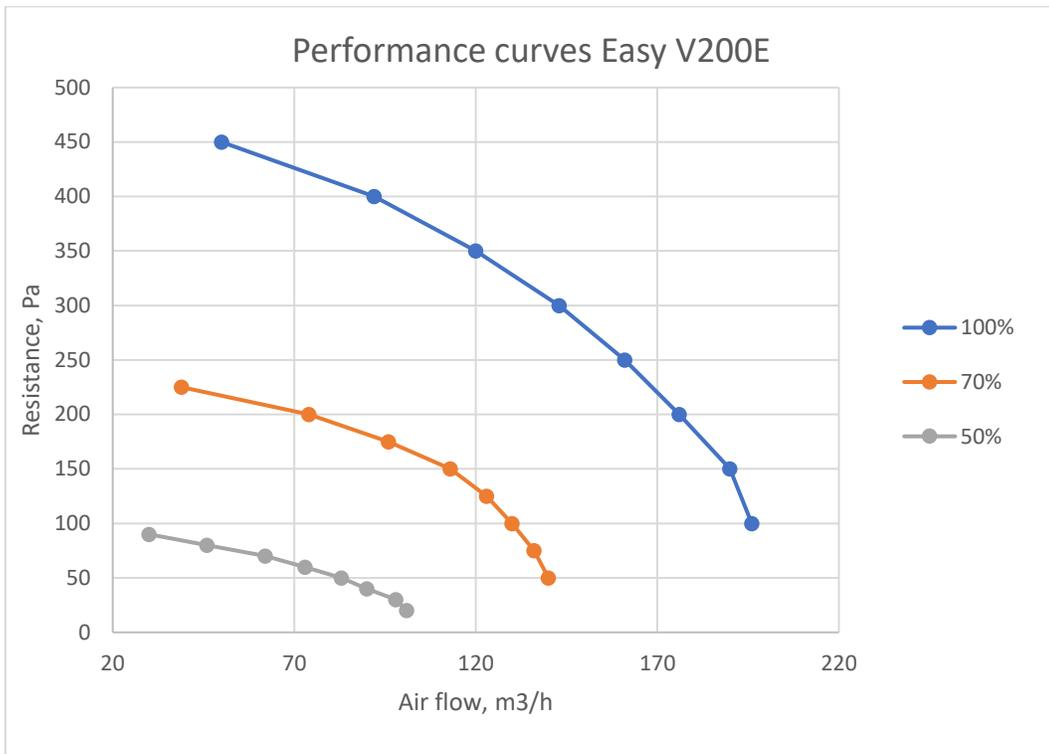
Graph 1 Dependence of ventilation power on the resistance of the installed ventilation system
