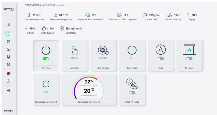
**Unit state** - Turning the device on / off
