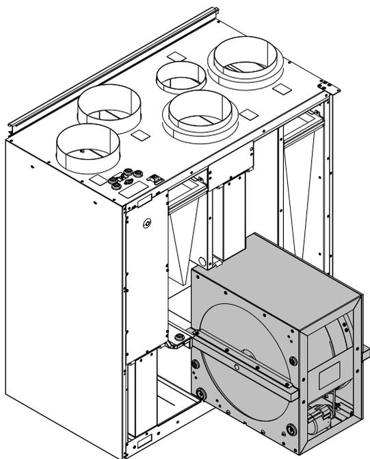
**Fig. 2 Heat exchanger**
