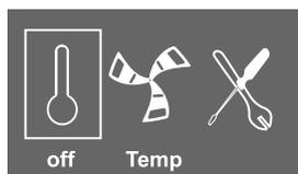
If the electrical re-heater is activated, it will switch off during manual summer mode. Manual summer mode goes automatically to step 1 (setpoint 12 °C) after two minutes if the supply air temperature is +5 °C or below.
