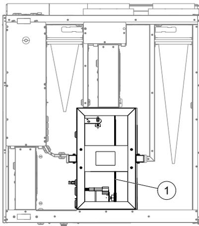
**Fig. 4 Rotor drive belt**
