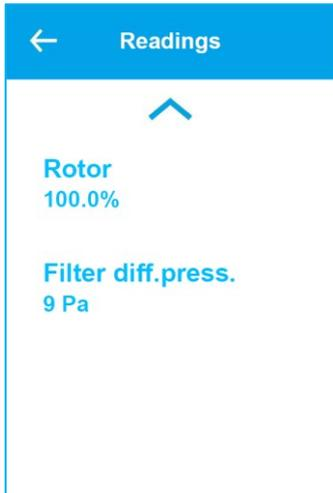
Speed of rotor heat exchanger
