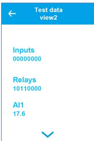
Show the digital inputs DIN1,2,3,4 – rest unused DIN1,2 NO; DIN3,4 NC
