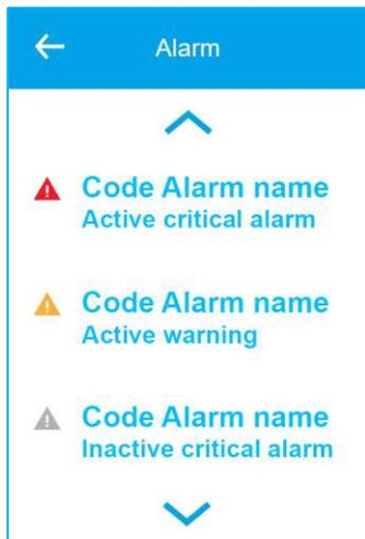
Sub-menu with warnings and critical alarms for the air handling unit.
