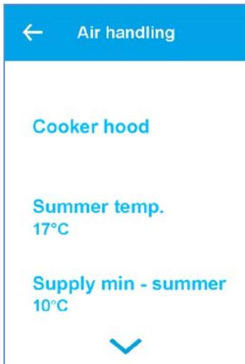
Sub-menu for configuration of the cooker hood function. The air handling unit will help push the steam towards the cooker hood
