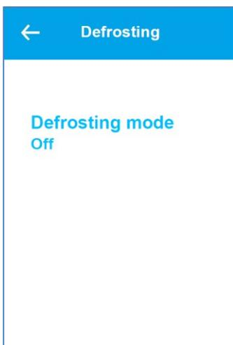
Defrost is done 6 min every hour by stopping supply fan and air heater. Exhaust fan set 30% and rotor at normal speed. Condition to start defrosting are the 3 modes.
