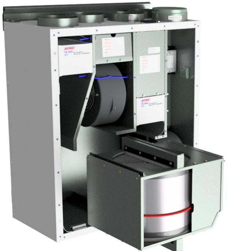
Rotor exchanger can easily be removed for cleaning, depending of AAHU model by unscrewing the 12 or 14 screws that holds it together.
