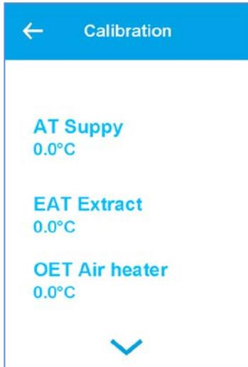
Menu for calibrating / offsetting the temperature sensors
