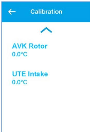
Adjust the AVK Rotor temperature sensor Range -5.0° .. +5.0°; default 0.0°
