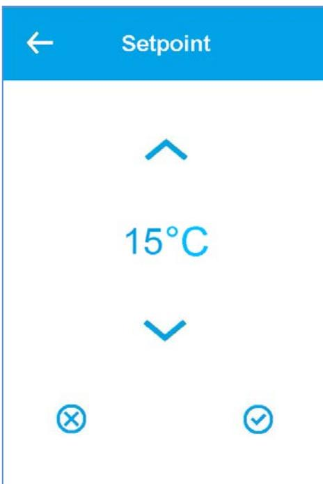
This will give you the possibility to change the temperature value in less than **10 seconds** by pressing ^ or v depending on your case. Accept the new set point value.
