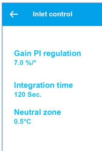
Inlet temperature controller gain Range 0%/° to 30 %/°
