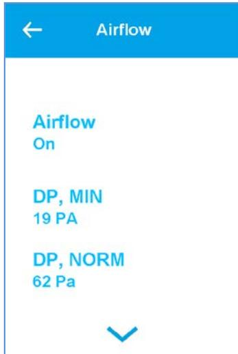
Settings for the air flow pressure sensor for the filter monitoring.
