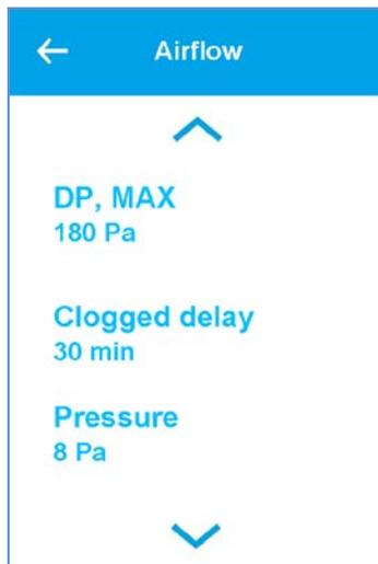
Maximum allowed pressure drop limit at MAX fan speed
