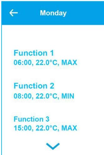
Every function or profile has its own 3 settings: Start time, set point and fan speed. When start time is reached, the set point is set to the entered value and fan speed to the setting
