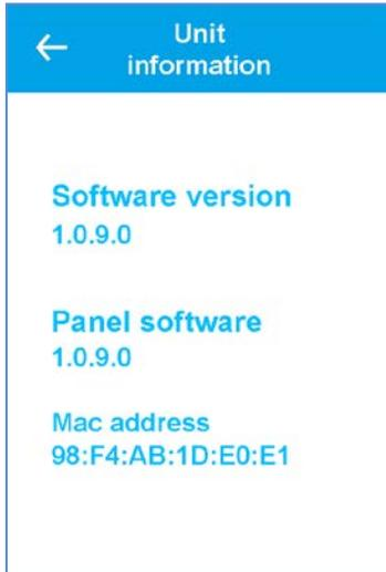
List the software versions in the controller and display of the air handling unit
