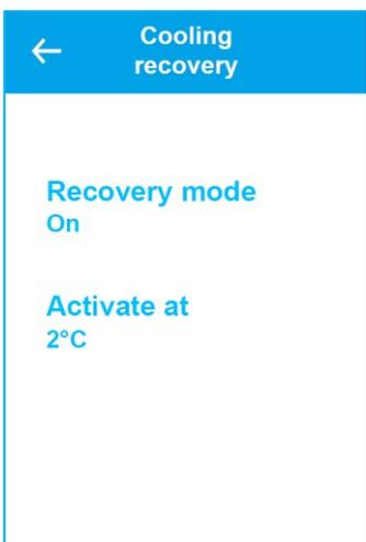
Cooling recovery is used when the intake air temperature is higher than the room temperature to keep the rooms cool.
