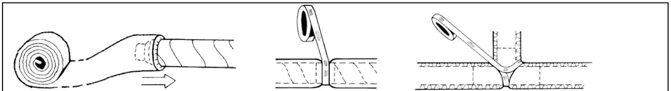
**Fresh air and exhaust duct should always be condensation insulated throughout its length.**
