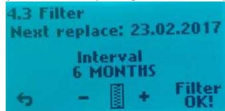
Alarm reset elapsed period by pressing the menu button 4, under "Filter OK"
