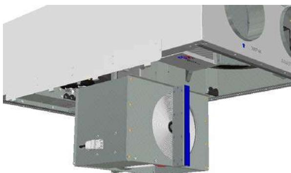
Rotor exchanger can easily be removed for cleaning by unscrewing 12 screws that hold it together.
