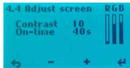
You can also adjust how long it should be light in the display after the operation.
