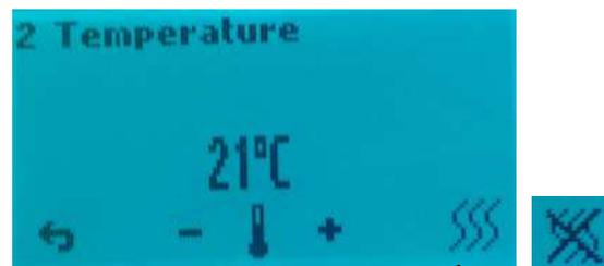
Indicator for activated heating coil. Small picture show not activated.
