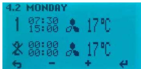
Choose airflow (fan speed) Speed dialing - **MIN** when one fan blade on the indicator is black. **NORM** = two black fan blades on the indicator. **MAX** speed = three black fan blades on the indicator.
