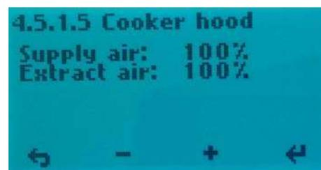
Supply and Extract air should have the same value as the MAX value under 4.5.1.3 (Set to 100% from factory.)
