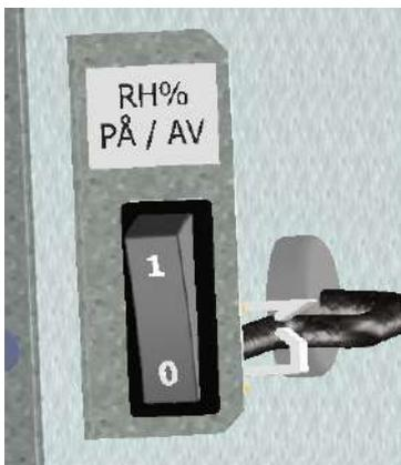
After startup, where the unit is placed into a new building with high humidity, you can let this humidity sensor be turned off for a period to avoid the full speed of the fan at night. To get the humidity sensor to operate as intended, you need at one time to put it active. Than you need to set the switch in position "1".
