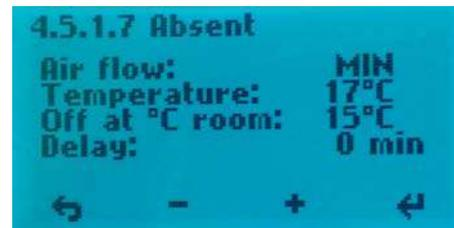
Set value of the desired temperature will show in the display after activating the function.
