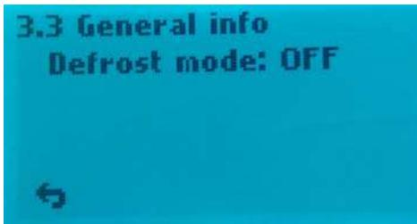
The unit is set in mode **OFF** from factory. If it is needed to change the defrost mode to another mode then press button 4 and scroll down to Configuration with button 3.
