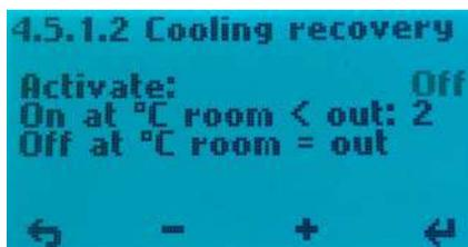
It is pre-programmed two options for use when the outside temperature is higher than the indoor temperature, heat recovery system will activate the function start and supply air will be cooled by exhaust air. Engagement when the outdoor temperature is 2 °C or 3 °C higher than room temperature. Use button 4 to change setting for Off. Press + to activate (On). Use button 4 to change setting for 2°C. Press + to change to to 3°C, if wanted.
