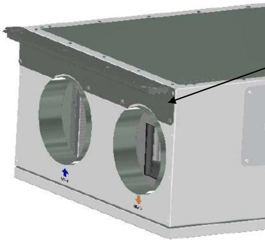
Suspension brackets screwed on the unit as shown on both ends of the unit.
