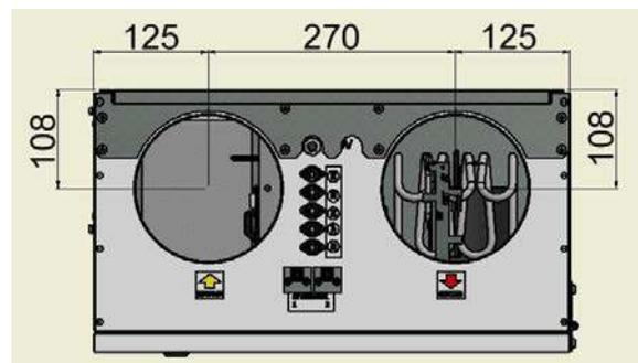
All ducts are  $\varnothing 160$  except the one for cooker hood that is  $\varnothing 125$  mm.
