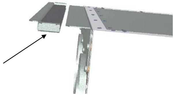
Attach one of the ceiling brackets in correct position in the roof.
