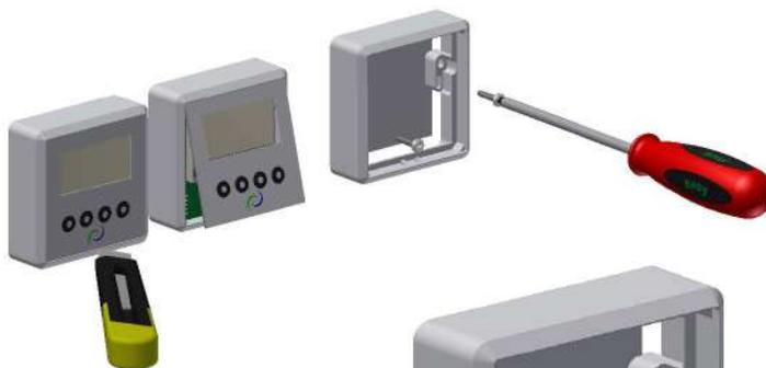
In order to dismantle the "touchpad" disc and display this can easily be done by using a knife with thin blade gently inserted between the jacket and the front plate. Then flip the knife down so that the frame loosens.
