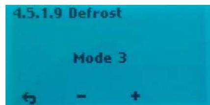
The function when defrosting starts is that each hour the supply air fan stops for 6 minutes. The heater **EV** turns off. Extract air fan reduces speed to 30% and the rotary exchanger will run as normal.
