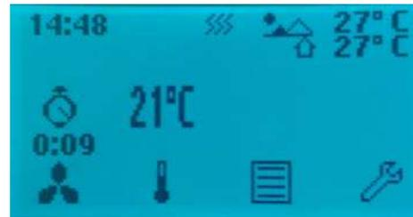
You can see that the fan are running with Max speed and the clock will start countdown. You can easy deactivate the fan boost again before the countdown automatically stops it.
