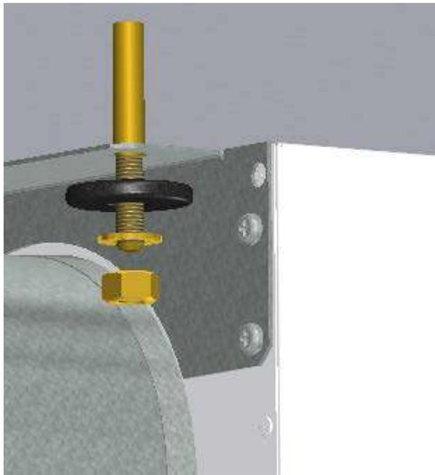
Make sure the bolt is turned so hard that it can not loosen. The bolts are available in different lengths so select someone suitable for this purpose. Lift the unit into position. Use a rubber cushioning, 4-6 mm thick, between washers and mounting brackets.
