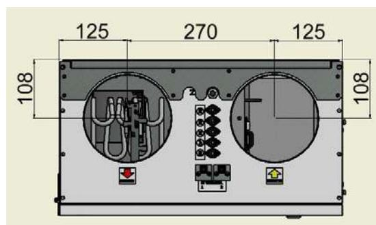
All ducts are  $\text{Ø}160$  except the one for cooker hood that is  $\text{Ø}125$  mm.
