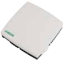
**Humidity sensor** (art.no. 110987) in both bathroom and wet room sends a signal to the unit to increase ventilation to max setting. The sensor has mechanical regulation and require control cable between sensor and unit. Multiple sensors - paralleled connection.
