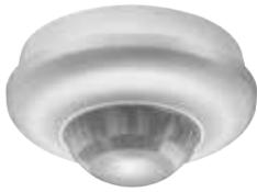
**Motion sensor** (art.no. 09390) in living room sends a signal to the unit to increase ventilation to max setting. Requires 230V operation voltage and control cable between sensor and unit. Multiple sensors - paralleled connection.
