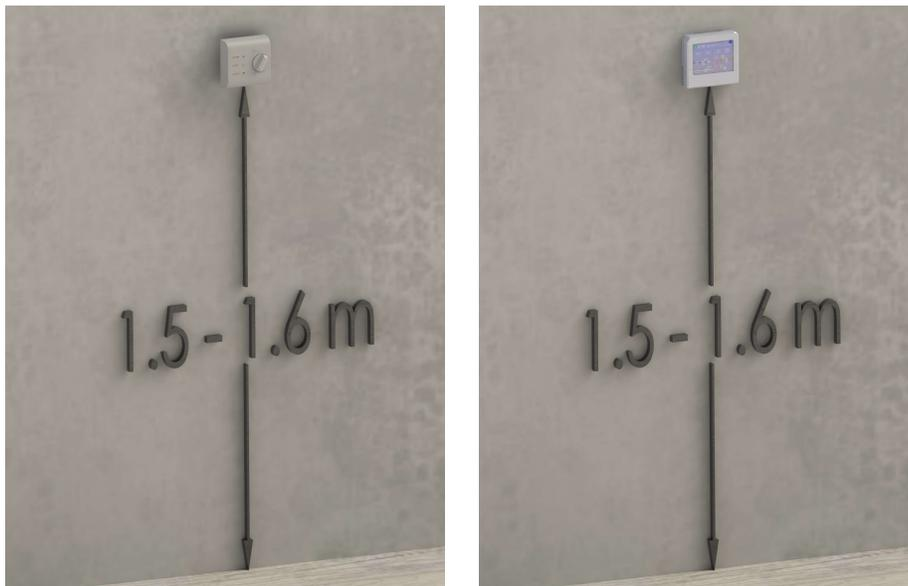
Figure 6. Installation of the control panel
