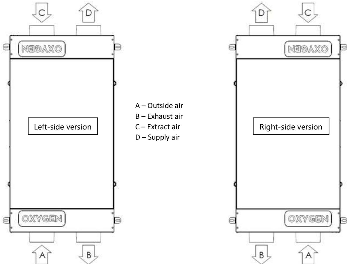
Figure 2. Mounting orientation
