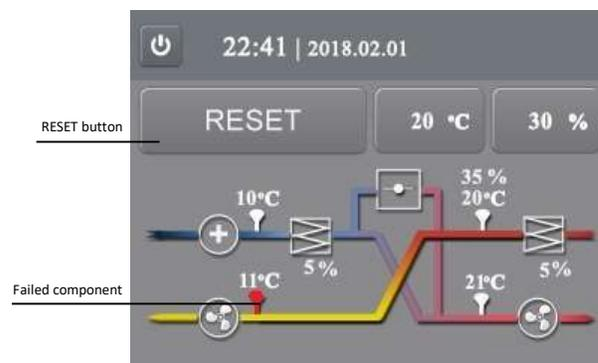
Figure 23. Failure indication
