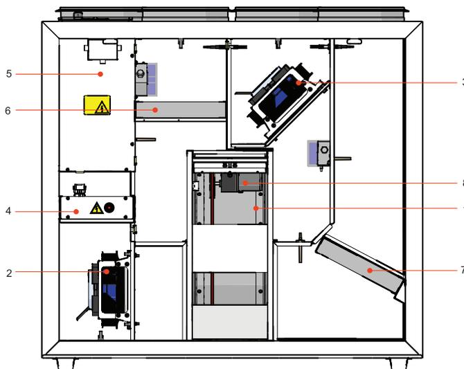
1 - Rotor heat exchanger; 2 - Supply fan; 3 - Exhaust fan; 4 - Electrical heater; 5 - Control board; 6 - Extract air filters (panel); 7 - Supply air filter (panel); 8 - Rotor motor.
