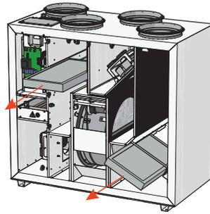
In order to remove the filters, open unit door and take off the filters.
