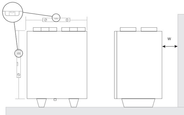
*Horizontal floor-mounting positions on floor (W=400 mm)*
