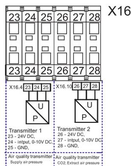
These sensors are intended for the following 3 functions: supply air pressure, extract air pressure and extract CO<sub>2</sub> detection. Supply air pressure is measured inside the supply air duct referenced to the unit's surrounding area. Extract air pressure is measured inside the extract air duct referenced to the unit's surrounding area. The CO<sub>2</sub> transmitter is installed in the extract air duct or room.
