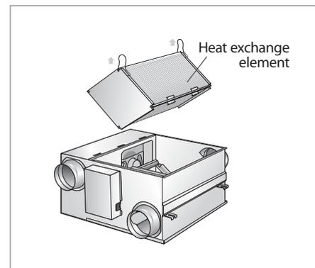
5. Reassemble the heat exchange element and the maintenance cover.
