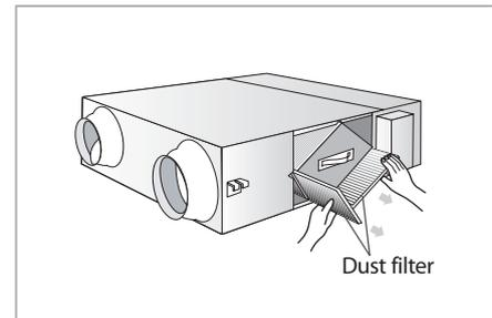
4. Remove all dust on the dust filters with a vacuum cleaner or a brush.
