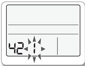
4. Press the  $\wedge$  or  $\sphericalangle$  button to select no.1
