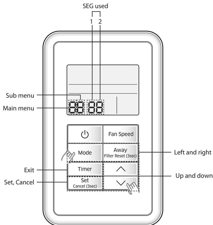
1. If you want to use the various additional functions for the ERV wired remote controller, press the Mode and  $\wedge$  buttons at the same time for more than three seconds.
