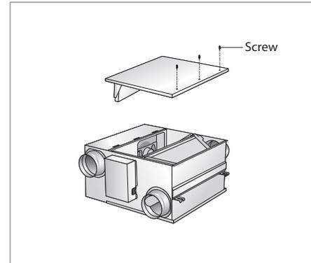
4. Remove all dust and particles on the heat exchange element with a nozzle of a vacuum cleaner.
