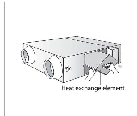
5. Reassemble the heat exchange elements and maintenance cover.
